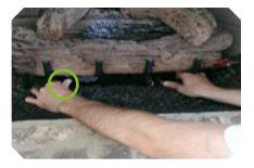
With the knob pushed in, press the igniter located on the extreme left side until the pilot light is lit.
