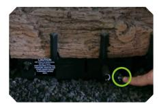
Turn the ON/OFF/PILOT knob on the right side to Pilot position. Once the knob is in the pilot position, push the knob forward. This will allow gas to flow to igniter.
